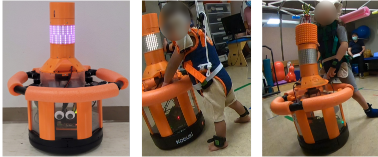
Fig. 1: GoBot, a custom assistive robot, during interactions with children with motor disabilities.
