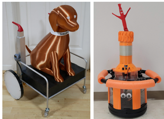
Fig. 1: Left : Shelbytron, a custom mobile assistive robot with light, joke, encouraging phrase, and music stimuli. Right : GoBot, a custom mobile assistive robot with light, music, and air dancer stimuli.
